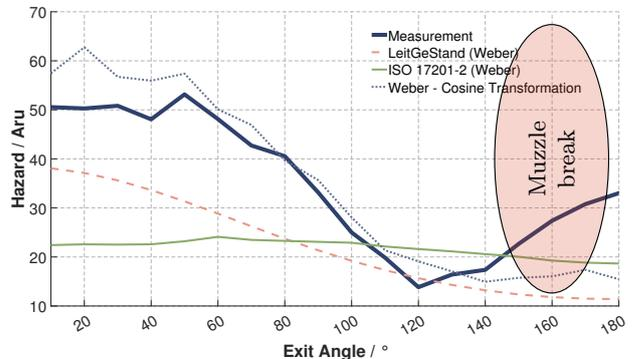
**Figure 6:** hearing load above the angle of exit<sup>2</sup>
