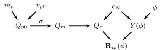
Figure 4: Reduced flow chart for calculating the Weber radius according to ISO 17201-2 (Fig. 2)
