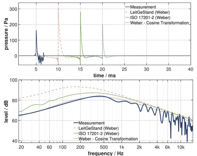
**Figure 9:** Sound pressure time curve and frequency response under  $130^\circ$  at 10 m distance
