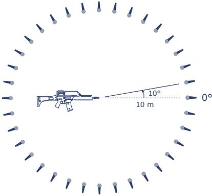
Figure 3: Sketch of the measuring points
