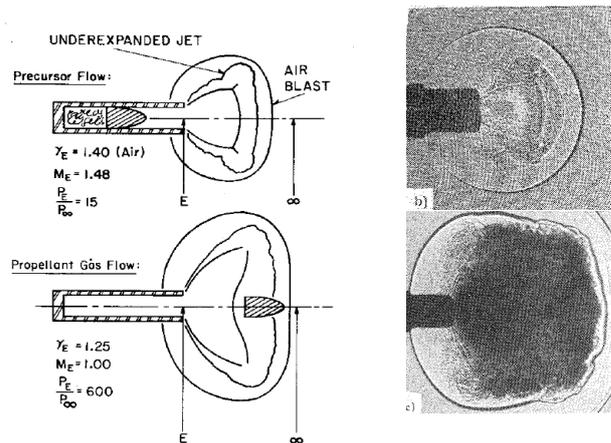
**Figure 2:** Flows occurring during the muzzle blast [5]
