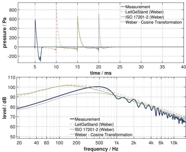
**Figure 7:** Sound pressure time curve and frequency response under  $10^\circ$  in 10 m distance
