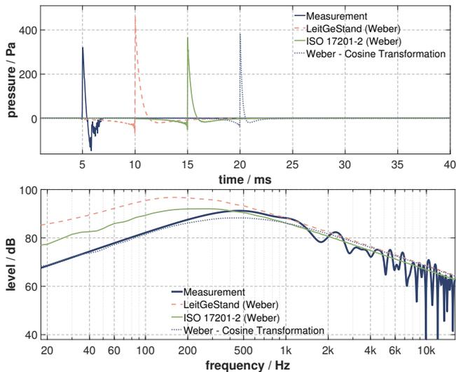
**Figure 8:** Sound pressure time curve and frequency response under  $90^\circ$  at 10 m distance
